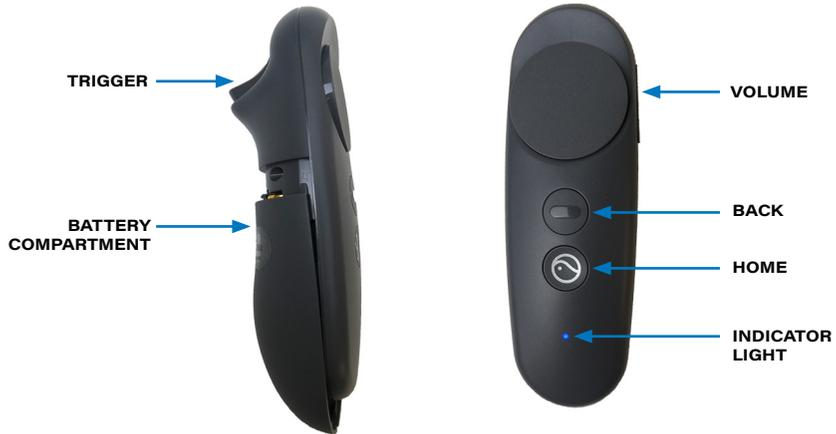
The controller is what you use to point and click in VR, using the trigger.
