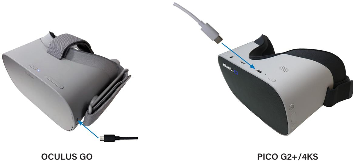
Headsets need about 2 hours to reach full charge. When the headset is at 90% battery, the indicator light next to the power button turns green.
